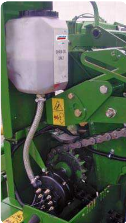
Agricultural machine (baler) with MOS/MOP 212 lubrication system
